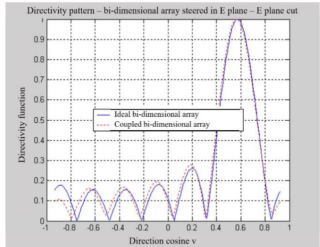
Figure 12. 7 by 7 planar finite array E plane steered directivity pattern – E plane cut
