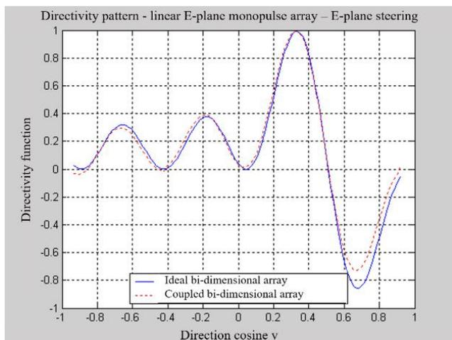
Figure 14. Pattern of a steered 8×8 E-plane monopulse array
