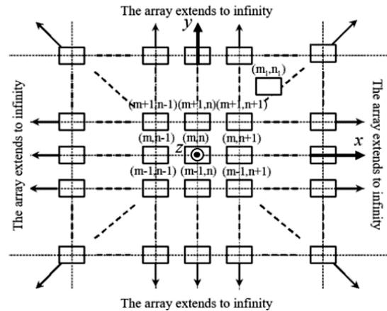
Figure 1. The topology of the infinite array. The elements are uniformly distributed in the  $(x,y)$  plane. The distances between the rows are  $D_x$  along the  $x$  axis and  $D_y$  along the  $y$  axis, respectively
