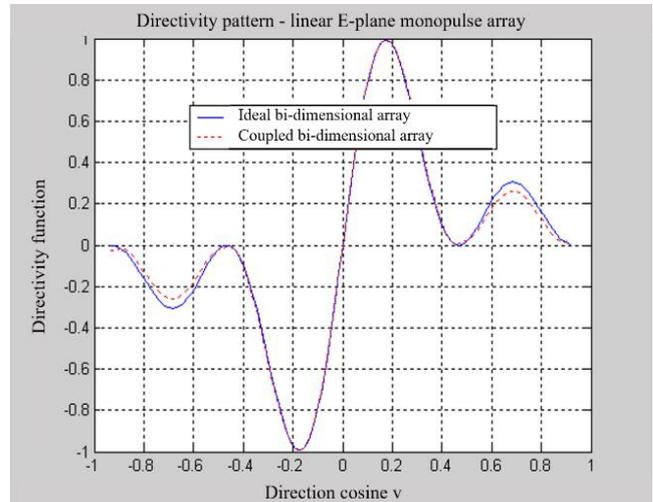
Figure 13. Pattern of an 8×8 E-plane monopulse array. The case of in-phase excitation
