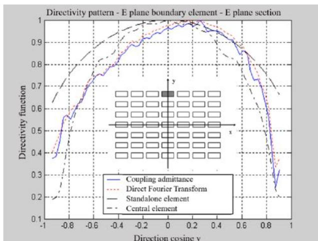
Figure 7. 21 by 21 planar finite array E plane boundary element directivity pattern – E plane cut, calculated by the methods of Coupling Admittances and Direct Fourier Window
