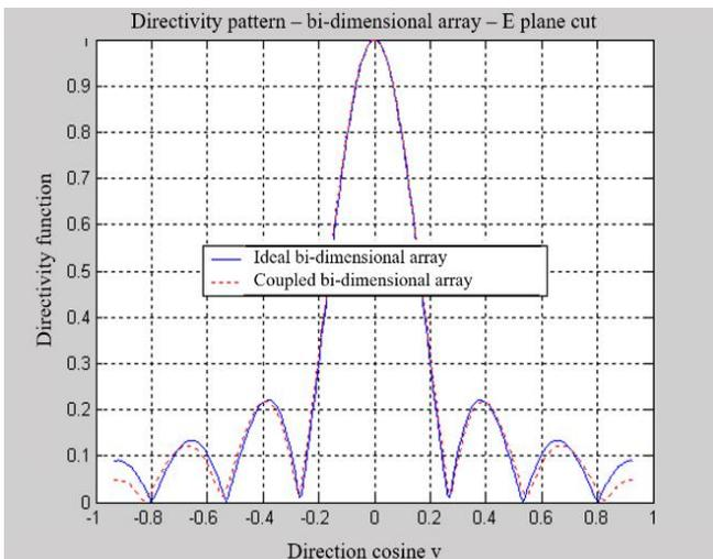
Figure 11. 7 by 7 in-phase planar finite array directivity pattern – E plane cut
