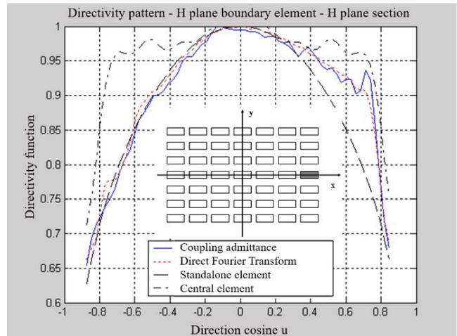
Figure 8. 21 by 21 planar finite array H plane boundary element directivity pattern – H plane cut, calculated by the methods of Coupling Admittances and Direct Fourier Window
