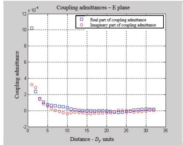
Figure 3. E plane cut (y axis) values of the real and imaginary values of the coupling admittances
