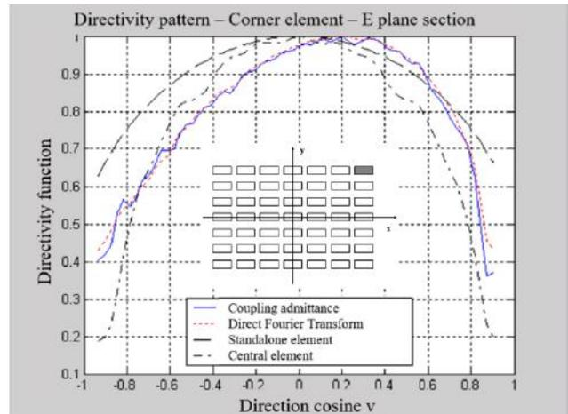
Figure 9. 21 by 21 planar finite array corner element directivity pattern – E plane cut, calculated by the methods of Coupling Admittances and Direct Fourier Window
