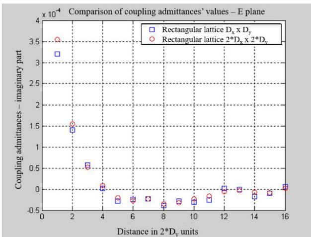
Figure 4. An E plane cut (y axis) comparison between the values of the coupling admittances of the original array and one with a double-size lattice
