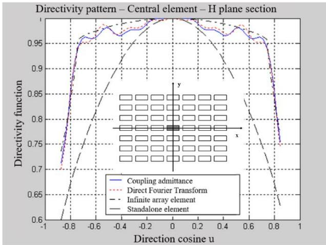
Figure 6. 21 by 21 planar finite array central element directivity pattern – H plane cut, calculated by the methods of Coupling Admittances and Direct Fourier Window
