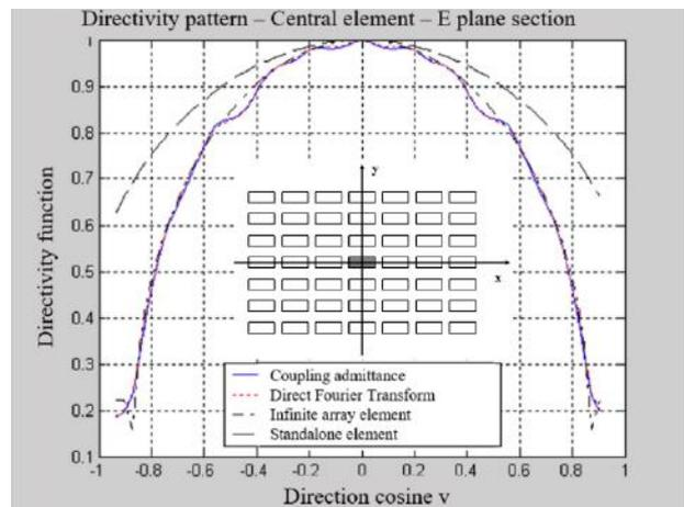
Figure 5. 21 by 21 planar finite array central element directivity pattern - E plane cut, calculated by the methods of Coupling Admittances and Direct Fourier Window
