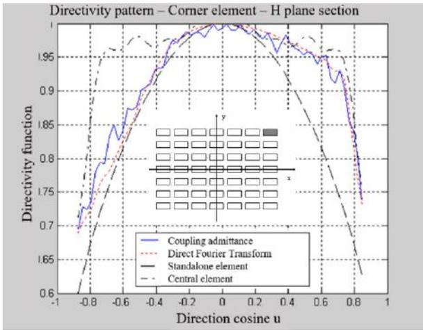
Figure 10. 21 by 21 planar finite array corner element directivity pattern – E plane cut, calculated by the methods of Coupling Admittances and Direct Fourier Window
