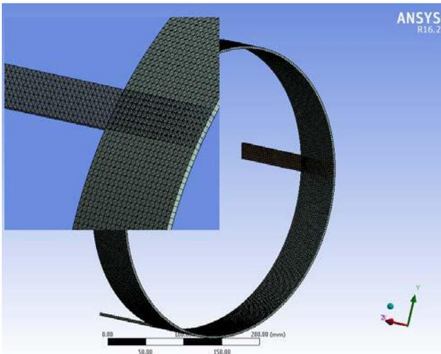
Figure 5. Meshing the duct with triangle elements
