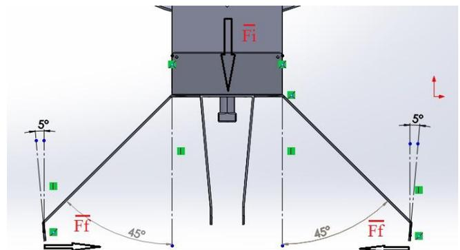
Figure 13. Bottom view of the paramotor frame
