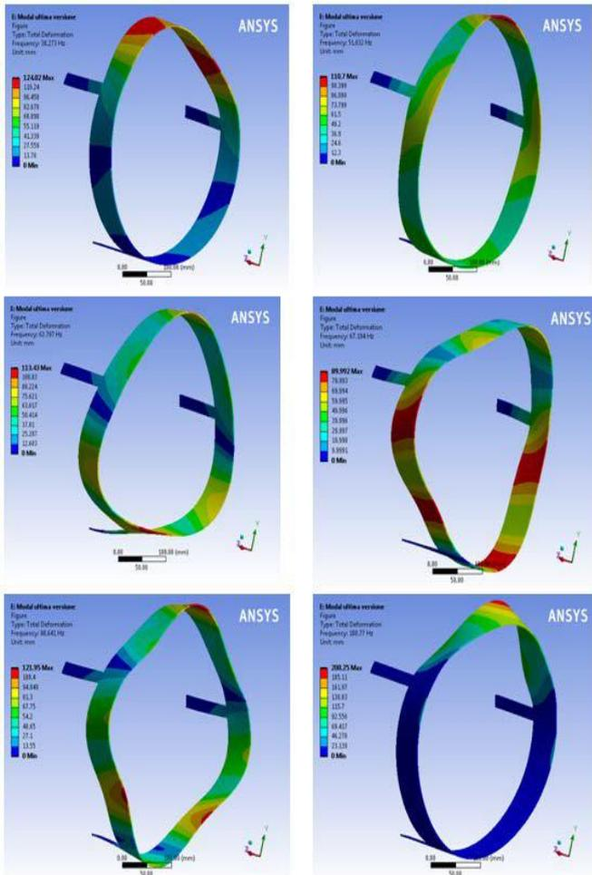
Figure 6. Mode shapes and natural frequency for the duct with Plexiglas material and aluminum alloy frame
