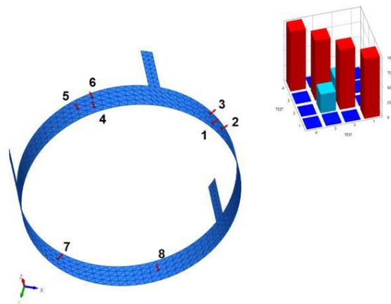
Figure 9. Positioning the 8 sensors using an auto generated stabilization chart (top right view) from the Femtools software
