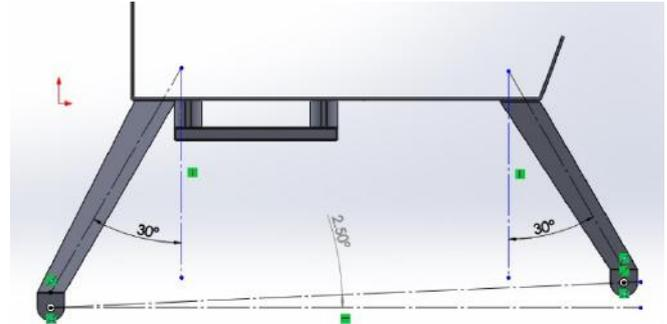
Figure 12. Landing gear angle modifications with respect to the vertical line
