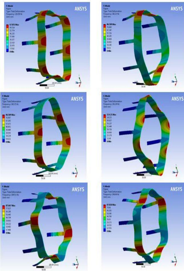
Figure 8. Mode shapes and natural frequency for the duct with Plexiglas material and aluminum alloy frame
