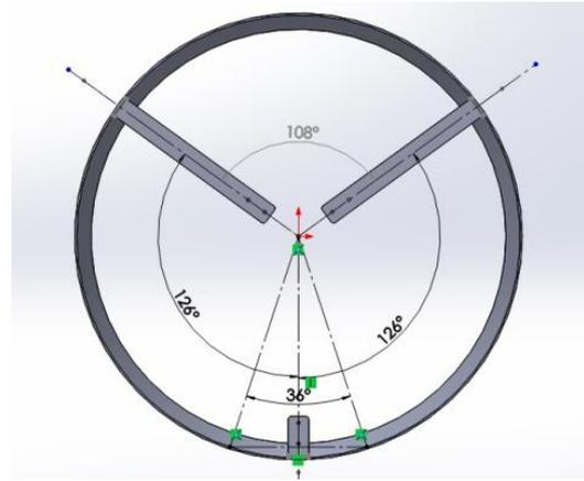
Figure 4. The tube fasten points locations
