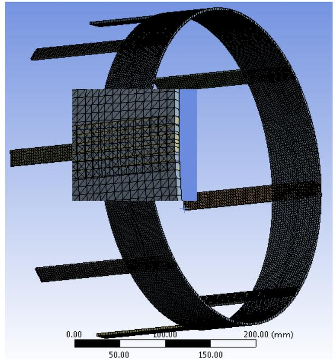
Figure 7. Meshing the improved duct with triangle elements and zoom in on elemental coupling
