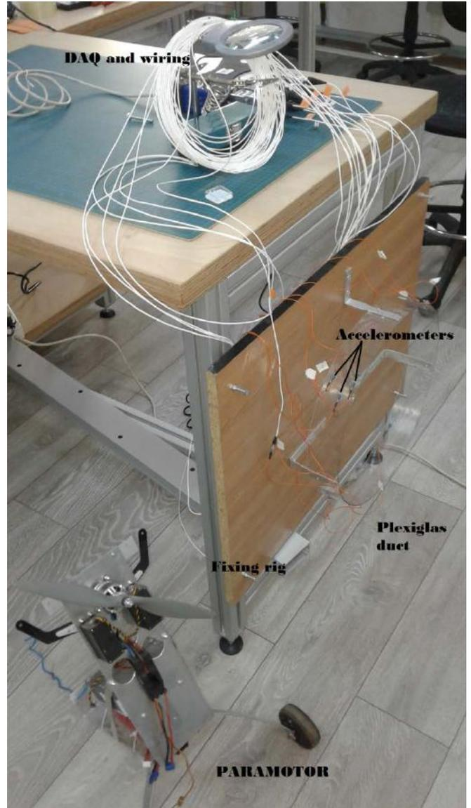
Figure 10. Experimental setup for modal analysis of Plexiglas duct with named components
