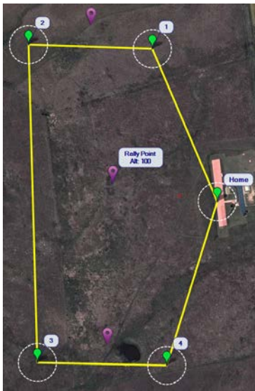
Figure 18. A flight plan with Rally Points. Rally Points are denoted with Purple place markers
