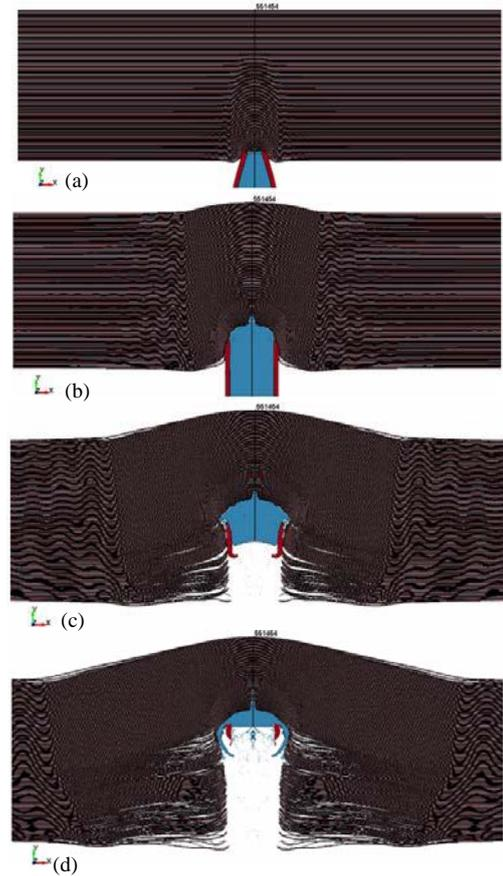
Figure 10. The evolution of the adhesive version of the UHMWPE ballistic impact problem – (a)  $t = 5\mu s$ ; (b)  $t = 20\mu s$ ; (c)  $t = 45\mu s$ ; (d)  $t = 65\mu s$
