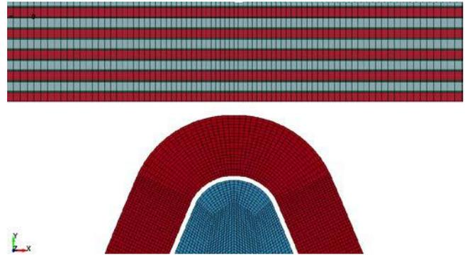
Figure 7. Discretization detail of the assembly, the adhesive version, impact zone
