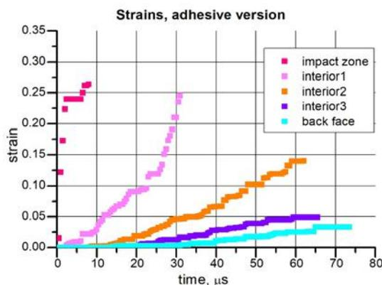
Figure 17. Strains in elements nearby the symmetry axis, adhesive simulation version
