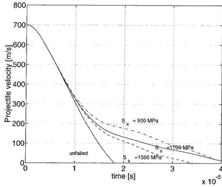
Figure 8. The velocity decrease of the projectile during the impact with an UHMWPE laminate panel [2]
