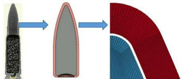
Figure 5. Graphical representation of the lead core 7.62×39 mm projectile
