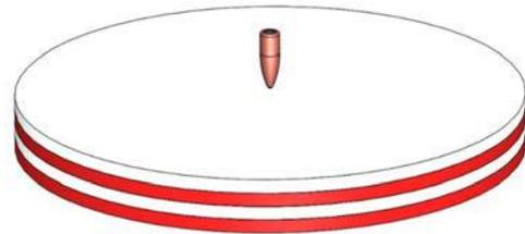
Figure 6. 3D schematization of the problem: the layout of the 7.62×39 mm, lead cored projectile and the Tensylon®-based composite target (the model is proportional, except for the thickness of the criss-cross layers, which are only illustrated to represent the orthotropic character of the material)
