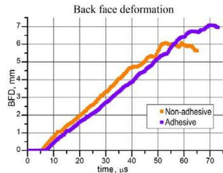
Figure 11. The back face deformation (BFD) evolution; the values represent the OY displacement of a chosen node, situated on the back face of the panel, close to the symmetry axis
