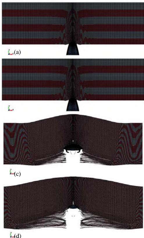
Figure 9. The evolution of the non-adhesive version of the UHMWPE ballistic impact problem – (a)  $t = 5\mu s$ ; (b)  $t = 20\mu s$ ; (c)  $t = 45\mu s$ ; (d)  $t = 65\mu s$
