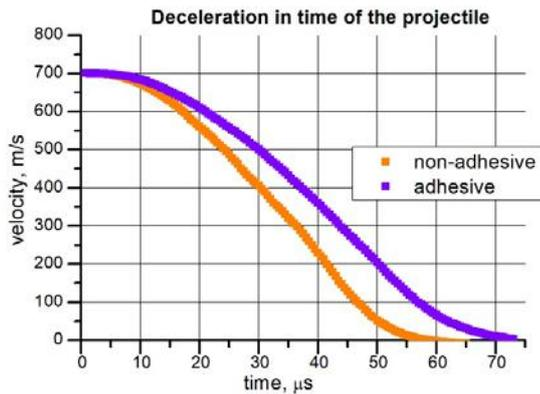
Figure 12. Deceleration of the projectile following the impact with the UHMWPE panel
