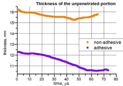
Figure 14. The evolution graph of the unpenetrated portion thickness
