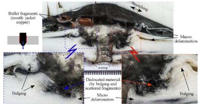
Figure 4. The penetration mechanisms in the Tensylon® panel
