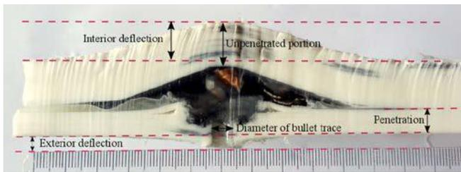
Figure 1. Significance of the measured dimensions in Table I
