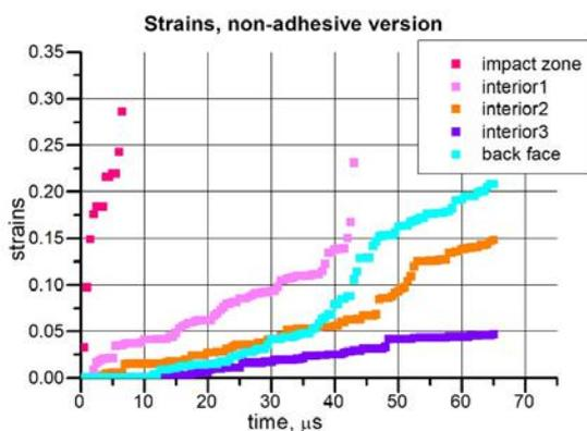
Figure 16. Strains in elements nearby the symmetry axis, non-adhesive simulation version
