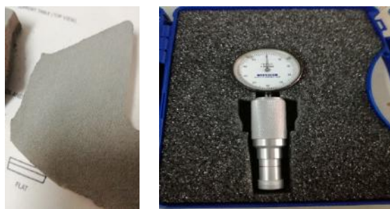
Figure 4. Propellant sample (left) and the Shore A durometer
