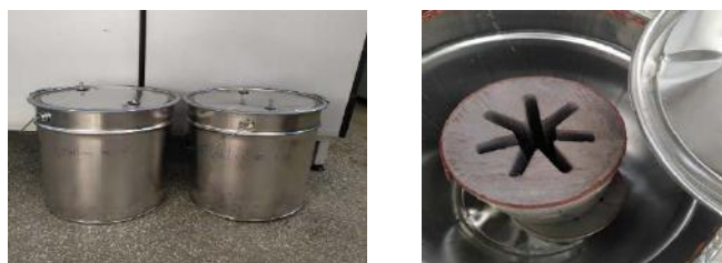
Figure 5. Preparation of propellant sample vessels for the ageing process
