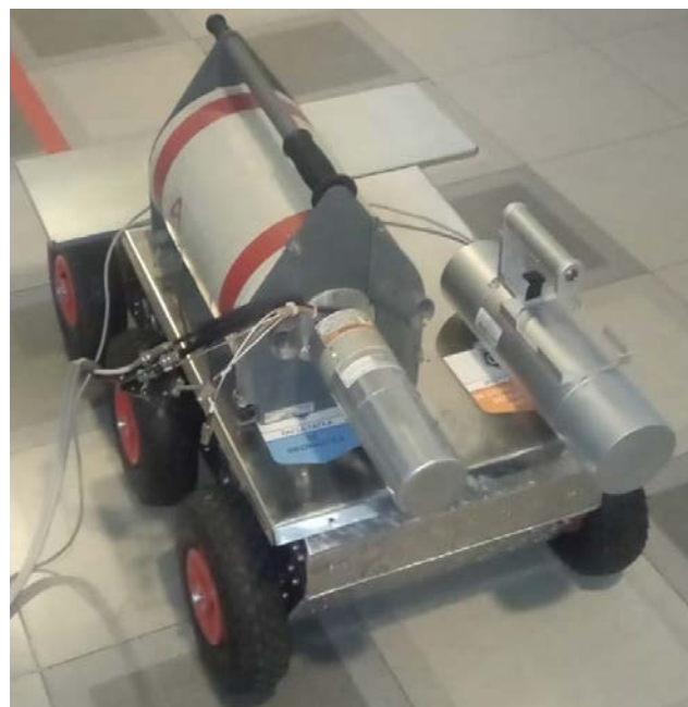
Figure 2. Example of a robot with six-wheel drive [3]
