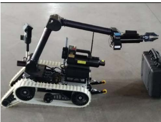
Figure 4. Example of a robot with a hybrid tracked propulsion system – https://www.army-technology.com/projects/cameleon-e-unmanned-ground-vehicle-ugv/
