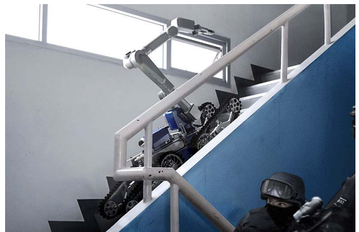
Figure 5. EOD Dual propulsion system robot – https://www.avinc.com/ugv/telemax-evo
