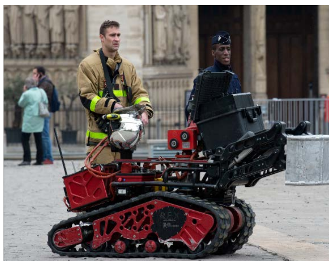
Figure 2. Colossus UGV manufactured by Shark Robotics used for extinguishing the fire at Notre Dames, Paris [8]
