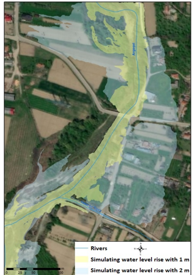
Figure 5. 2D water-level rise visualisation on the 1 m DTM (+1 m = yellow; +2 m = blue) overlaid on the orthophoto; encroachment concentrates along the Argeșel corridor and at the Valea lui Topor/Mâzgana confluences
