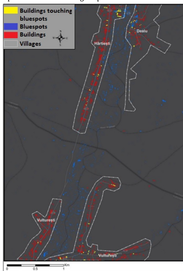
Figure 3. Baseline flood-susceptibility map: bluespots and buildings intersecting or adjacent to depressions in Hârtiești, Dealu, and Vulturești (Argeșel Basin)
