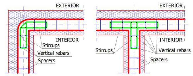
Figure 4. Intersection details for reinforced concrete walls
