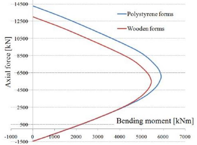
Figure 12. P-M interaction for reinforced concrete walls
