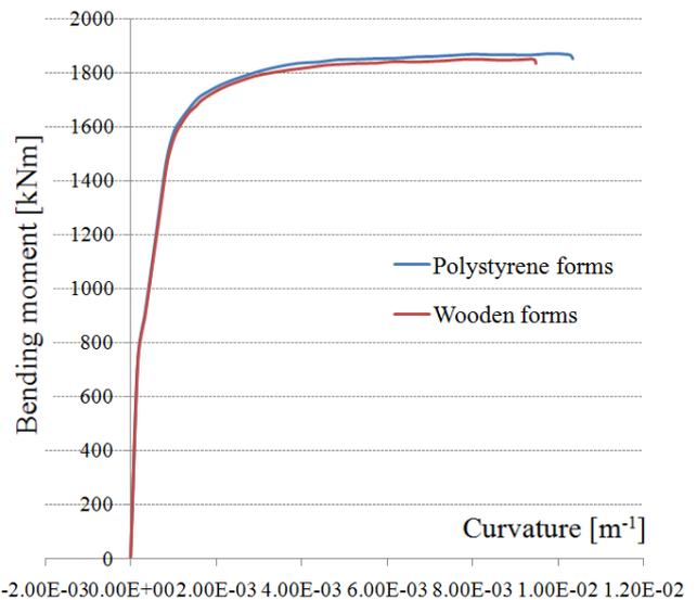
Figure 10. Bending moment - curvature relation
