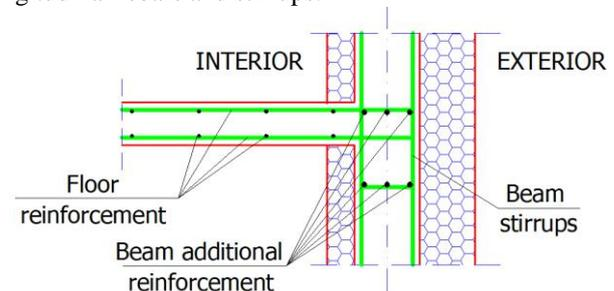
Figure 5. Detail of floor-wall intersection
