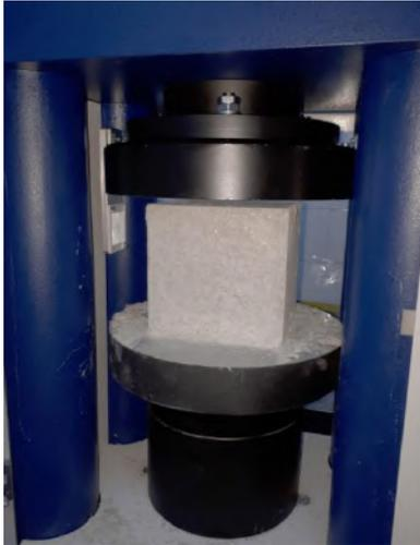
Figure 6. Testing the concrete specimens
