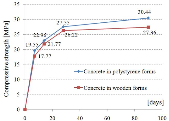
Figure 7. Values of compressive strength for concrete specimens tested after different storing intervals
