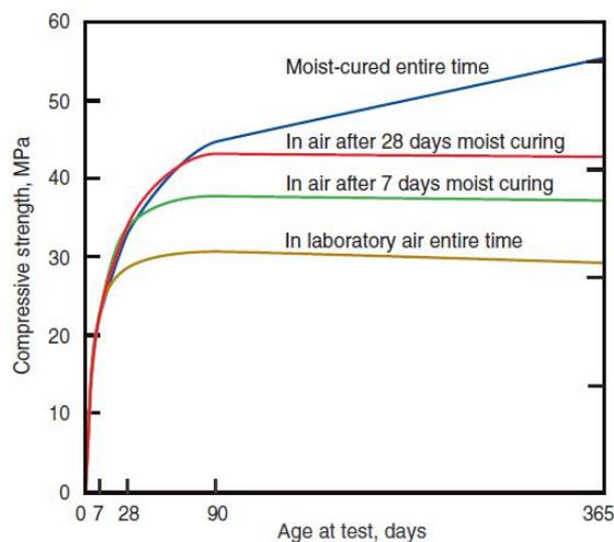
Figure 3. Effect of moist curing time on strength gain of concrete [5]
