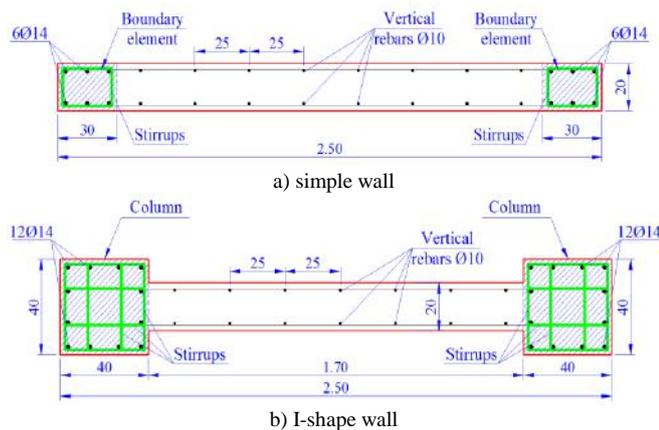
Figure 9. Types of concrete walls and reinforcement details
