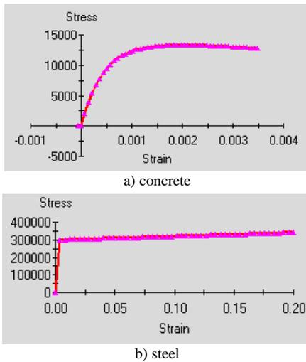
Figure 8. Constitutive laws for component materials of reinforced concrete element
