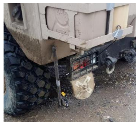
Figure 6. IL-600 sensor mounted at the rear part
