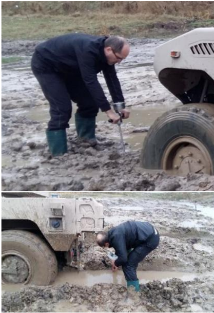
Figure 7. Cone Index and soil moisture measurements
