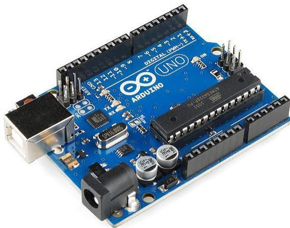
Figure 7. The Arduino UNO development board
