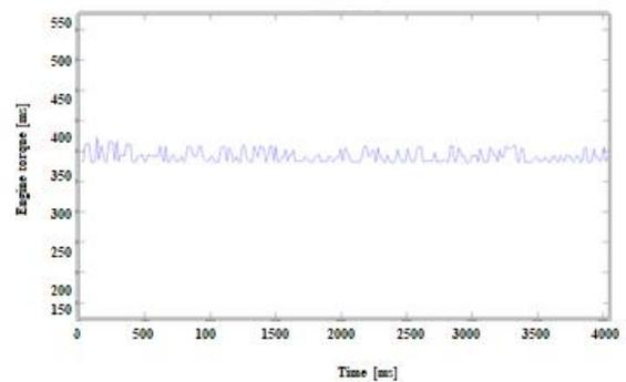
Figure 9. Time variation for engine torque corresponding to right wheel of rear axle
