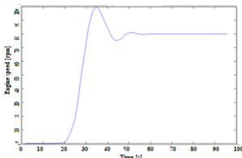
Figure 12. Time variation of engine speed
