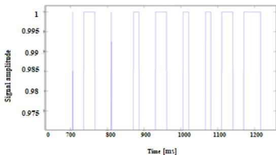
Figure 7. The signal originating from the encoder corresponding to the right wheel of rear axle
