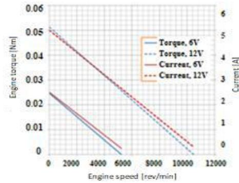
Figure 4. Revolution characteristics of electrical engine axle
