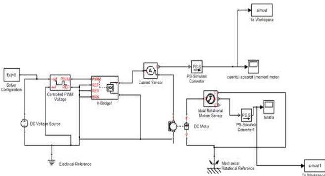
Figure 11. The measuring system in Simulink
