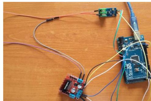
Figure 3. Current sensor attached to measuring system
