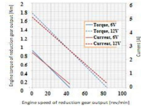
Figure 5. Revolution characteristics of reduction gear axle
