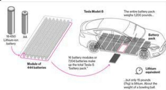
Figure 3. Power Cells for the Tesla Model S P85D Electric Car [3]
