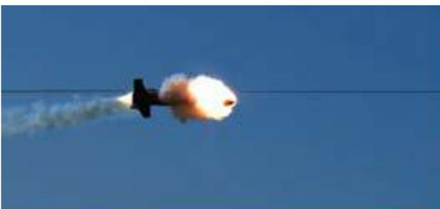
Figure 1. Inactivating a missile with a LASER beam [4]
