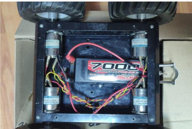
Figure 2. Power supply block
