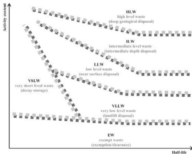
Figure 2. Radioactive waste classification scheme [29]
