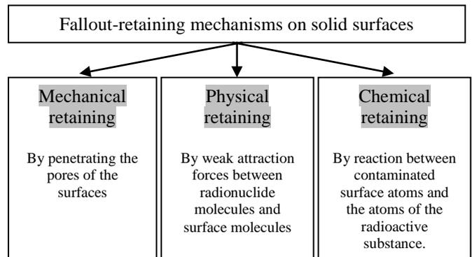
Figure 4. RWA interaction with surfaces
