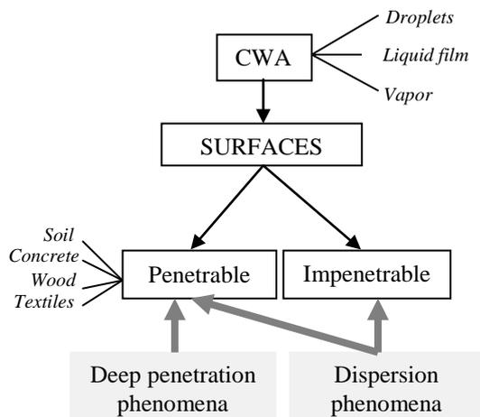
Figure 3. CWA interaction with surfaces
