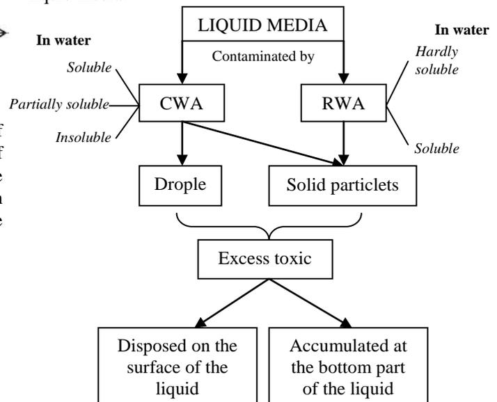
Figure 5. CWA and RWA interaction with liquid media
