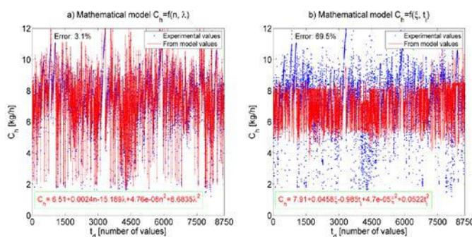
Figure 5. Establishing mathematical models based on information theory, for hourly fuel consumption 50 test runs of Logan Laureate vehicle
