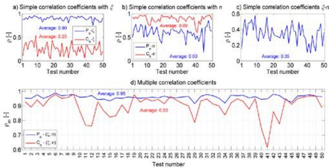
Figure 6. Values for simple and multiple correlation coefficients for engine output power and hourly fuel consumption, 50 experimental test runs, Logan Laureate Vehicle
