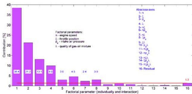
Figure 2. Study on the influence of certain factors over engine output power by applying generalized MANOVA algorithm, 50 experimental test runs, Logan Laureate vehicle.
