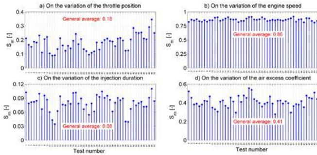
Figure 1. Average values for sensitivity function of hourly fuel consumption, 50 experimental test runs on Logan Laureate vehicle
