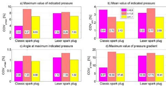
Figure 6. Coefficients of variation for maximum pressure, mean pressure, maximum pressure angle, pressure gradient, Dacia mono cylinder for: 50 cycles;  $n = 2800 \text{ rev/min}$ ;  $\kappa = 90\%$ ;  $\lambda = [0.9; 1.0; 1.1]$
