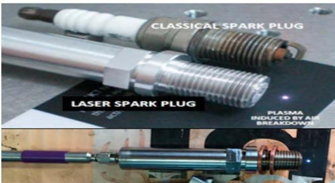
Figure 3. CFR Octane Rating Unit Engine equipped with LI
