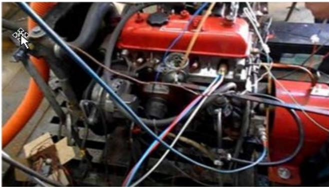
Figure 1. Dacia Single cylinder SI engine equipped with LI
