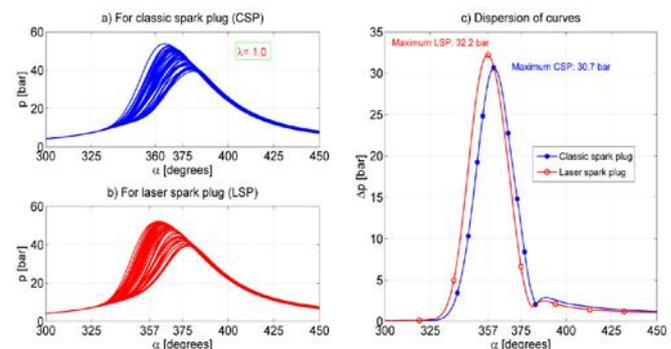
Figure 9. The indicated pressures and the dispersion of their curves (details), Dacia mono cylinder, for: 50 cycles;  $n = 2800 \text{ rpm}$ ;  $\kappa = 90\%$ ;  $\lambda = 1.0$
