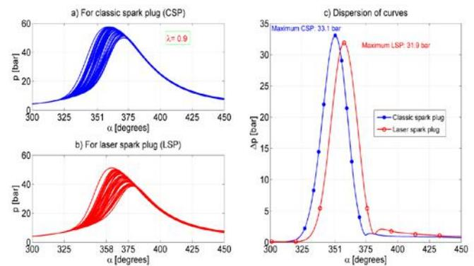
Figure 8. The indicated pressures and the dispersion of their curves (details), Dacia mono cylinder, for: 50 cycles;  $n = 2800 \text{ rpm}$ ;  $\kappa = 90\%$ ;  $\lambda = 0.9$
