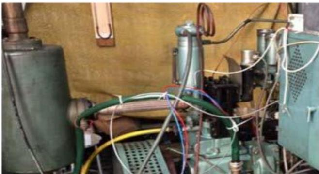
Figure 2. CFR Octane Rating Unit Engine equipped with LI
