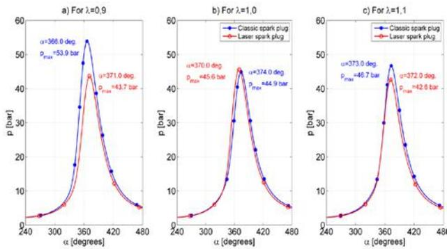
Figure 10. The indicated pressure for the Dacia single-cylinder curve for: 50 cycles;  $n = 2800$  rpm;  $\kappa = 90\%$ ;  $\lambda = [0.9; 1.0; 1.1]$
