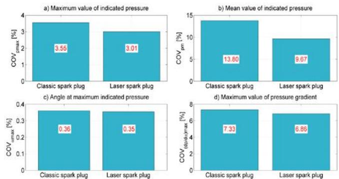
Figure 5. Coefficients of variation for maximum pressure, mean pressure, maximum pressure angle, maximum pressure gradient, CFR engine for: 491 cycles;  $n = 900$  rev/min;  $\beta = 28.5^\circ$  RAC;  $\lambda = 1.1$
