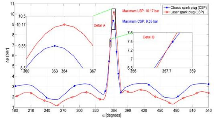
Figure 7. Dispersion of the cycle pressure curves for the classic spark plug and LI,  $\beta = 28.5^\circ \text{CAD}$ ,  $\lambda = 1.1$
