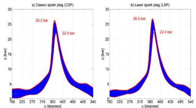
Figure 4. The indicated pressure, instantaneous values and cycle tires the CFR engine for 491 cycles,  $n = 400$  rev/min,  $\beta = 28.5^\circ$  RAC, and  $\lambda = 1.1$
