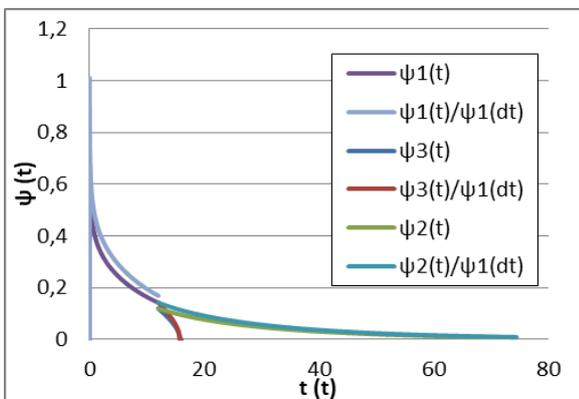
Figure 7. Comparison between the three-interval window-function  $\psi(t)$  and the function scaled to  $1\psi(t)/\psi1(dt)$  for the defining intervals 0-12 s, 12-16 s and 16-end. Number indices refer to the function branches and correspond to the order of parameter determination (1 - first interval 0-12 s, 2 – third interval 16-end, 3- second interval 12-16 s)
