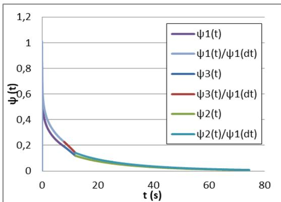
Figure 6. Comparison between the three-interval window-function  $\psi(t)$  and the function scaled to  $1\psi(t)/\psi1(dt)$ . Number indices refer to the function branches and correspond to the order of parameter determination (1 - first interval 0-8 s, 2 – third interval 12-end, 3 – second interval 8-12 s)
