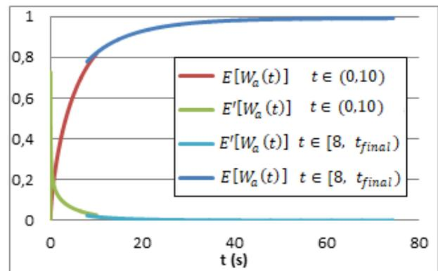
Figure 2. The expected mean square acceleration function defined on two intervals  $E[W_a(t)]$  and its derivative
