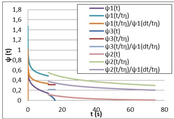
Figure 5. Comparison between the three-interval window-function  $\psi(t)$ , the function in normalized time  $\psi(t/t_n)$  and the function in normalized time scaled to  $1\psi(t/t_n)/\psi1(dt/t_n)$ . Number indices refer to the function branches and correspond to the order of parameter determination (1 – first interval 0-8 s, 2 – third interval 12-end, 3 – second interval 8-12 s)
