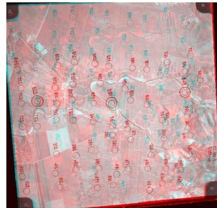
Figure 7. Stereo representation by the anaglyphs method of normalized aerial recordings
