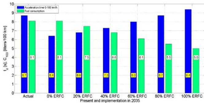
Figure 2. Forecast for 2035 for dynamics and fuel saving
