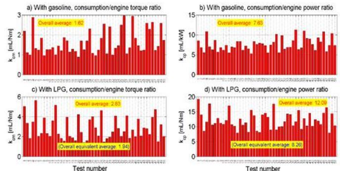
Figure 7. Average values/tests of energy efficiency criteria  $k_{cm}$  and  $k_{cp}$
