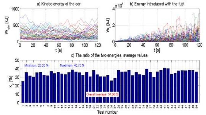
Figure 3. Criterion for energy efficiency  $k_c$  for operation with gasoline
