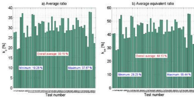
Figure 4. Mean of tests energy efficiency criterion  $k_c$  for operation with LPG
