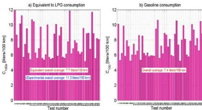
Figure 5. Fuel consumption per 100 kilometers on petrol and LPG operation
