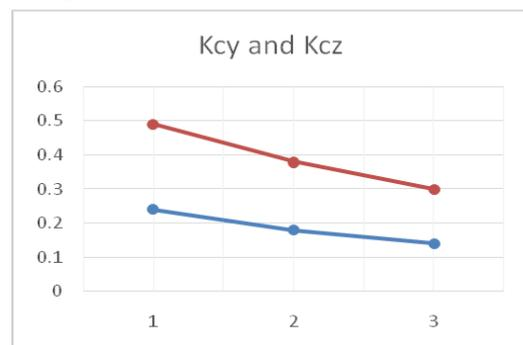
Figure 4. Representation of the buckling factors according to EC5 for the three column heights 3 m, 3.5 m and 4 m, on both y and z directions
