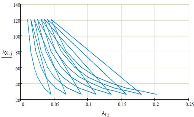
Figure 1. Representation of the slenderness coefficients on the y direction with respect to the area combinations, H = 3.5 m
