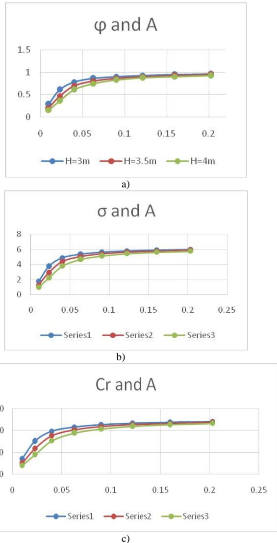
Figure 3. Representation of: a) the buckling coefficients; b) the compression stresses; c) the strength capacities for all the heights
