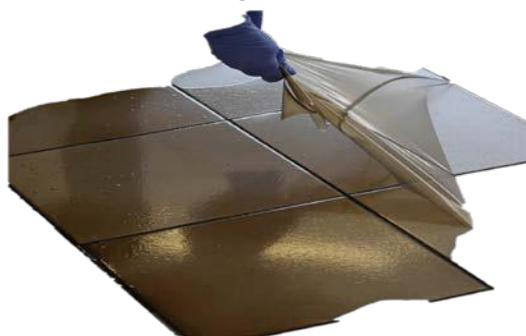
Figure 6. Peeling off the strippable coating from the surface
