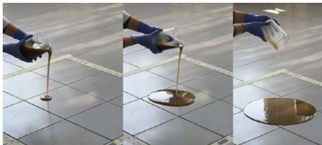
Figure 5. Pouring the decontamination solution over a specific area
