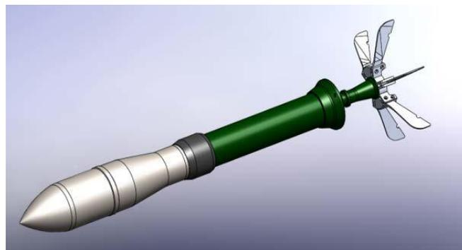
Figure 1. The warhead and the rocket motor of the ammunition, on the trajectory (without propellant charge and with opened stabilizing fins)
