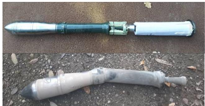
Figure 14. The ammunition before firing and after steel target penetration tests
