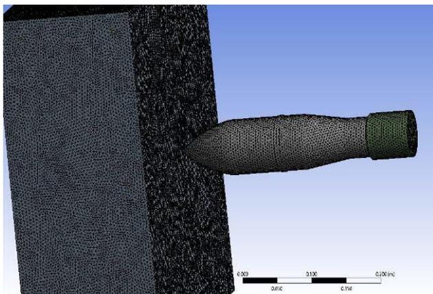
Figure 7. Model meshing of the impact between the projectile and 200 mm C35/C37 concrete double reinforced with rebar.
