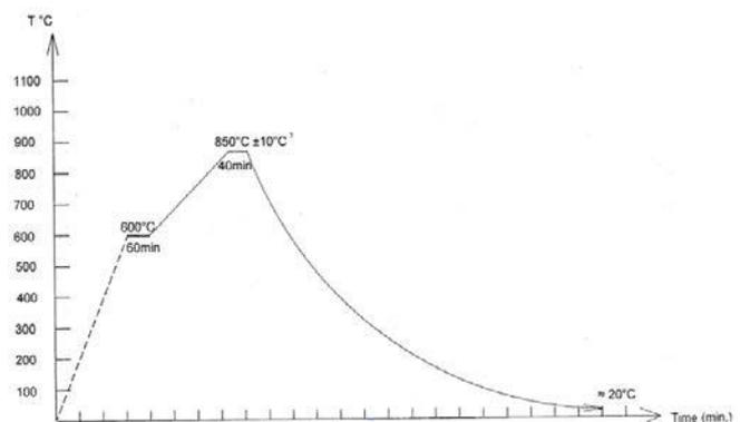
Figure 4. Thermal treatment diagram of 35HGSA hardened steel
