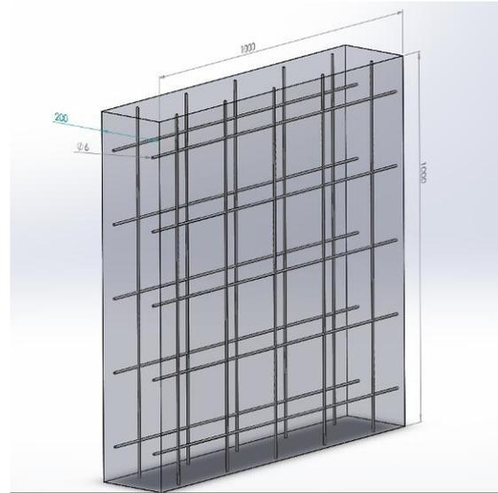
Figure 8. Detail on the model for 200 mm thick concrete target reinforced with 6 mm steel rebars
