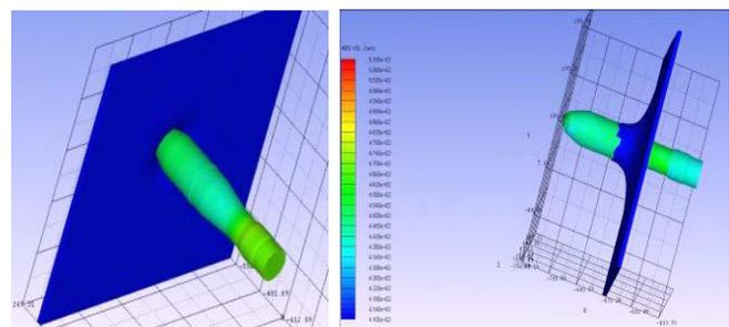
Figure 9. Numerical simulation of the impact between the projectile and the armor plate
