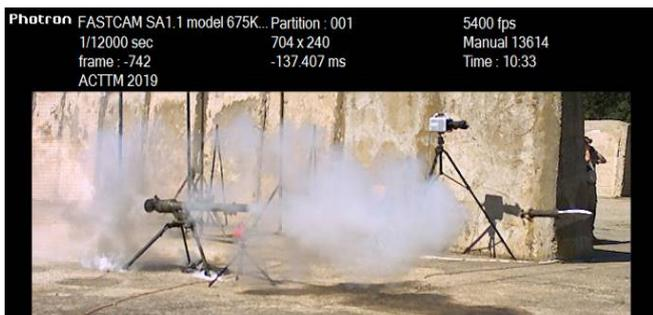
Figure 11. Live firing of the piercing ammunition with thermobaric effect
