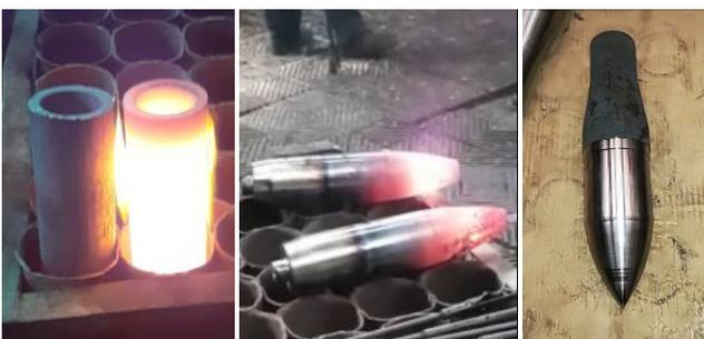
Figure 3. Different phases in the manufacturing process of projectile
