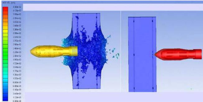
Figure 10. Numerical simulation of the impact between the projectile and the concrete target
