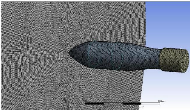
Figure 6. Model meshing of the impact between the projectile and 20 mm homogenous steel target.
