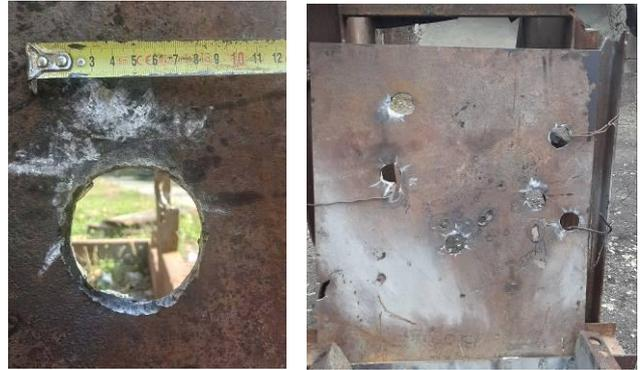
Figure 13. Homogenous steel armor penetration tests
