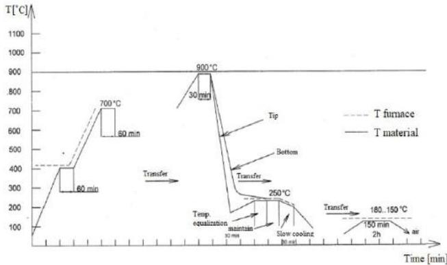
Figure 5. Final thermal treatment diagram of 35HGSA hardened steel
