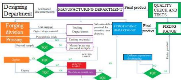
Figure 2. Schematic manufacturing process of the projectile
