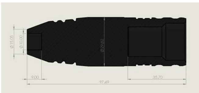
Figure 3. Model for hollow point shape configuration for AP-T projectile (section view)
