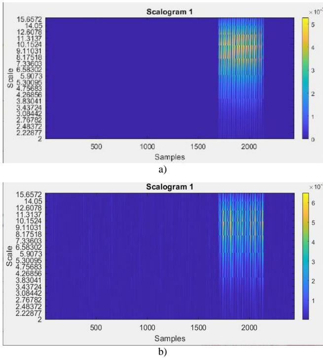
Figure 10. a) First ideal signal in the time domain and its scalogram using Haar Wavelet b) Noisy signal in the time domain and its scalogram using Haar Wavelet
