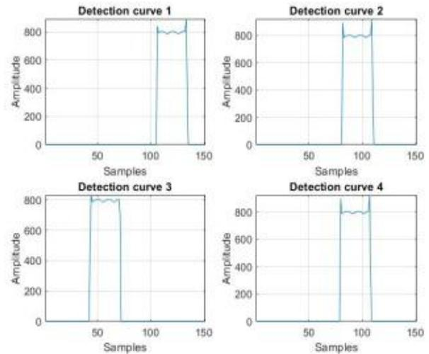
Figure 8. Detection curves for noisy signals in the case of the Spectrogram
