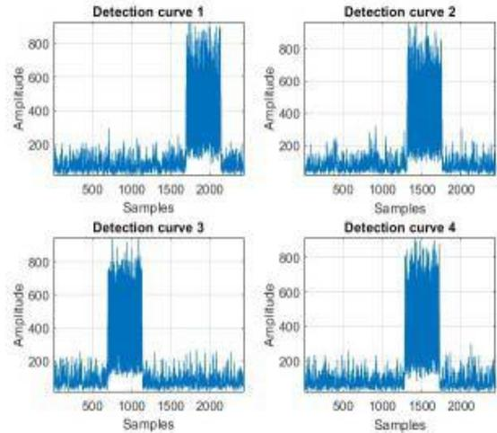
Figure 12. Detection curves of ideal signals in the case of Wavelet Transform
