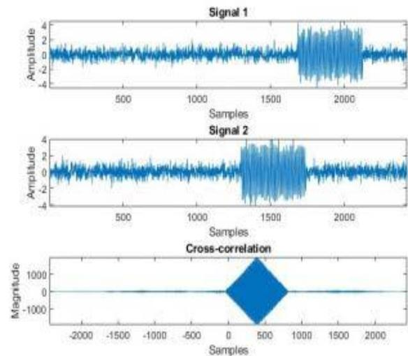
Figure 4. Graphical representation of the signals and the Cross-correlation
