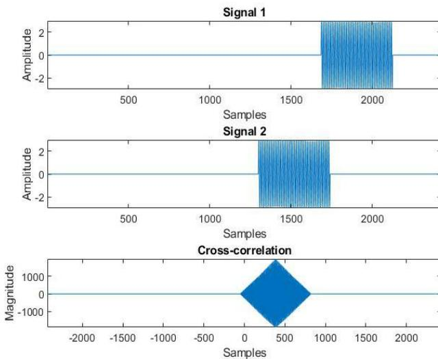
Figure 3. Graphical representation of the signals and Cross-correlation
