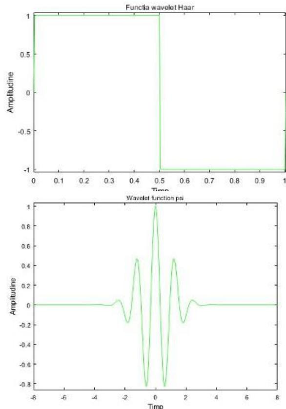
Figure 9. Graphical representation of Haar Wavelet and Morlet Wavelet in the time domain
