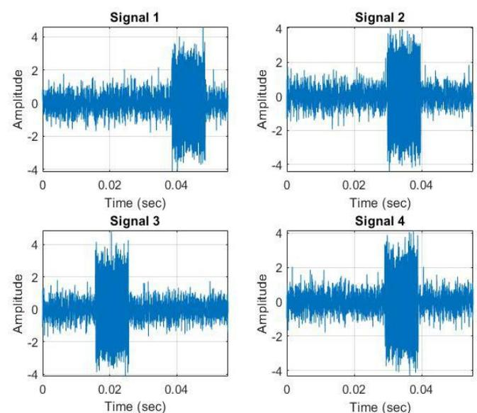
Figure 2. Signals with a SNR = 5 dB in the time domain
