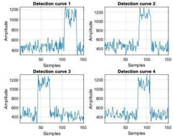
Figure 7. Detection curves for ideal signals in the case of the Spectrogram
