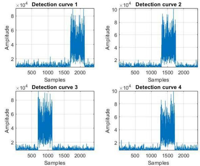
Figure 18. The detection curves of noisy signals in the case of RPA
