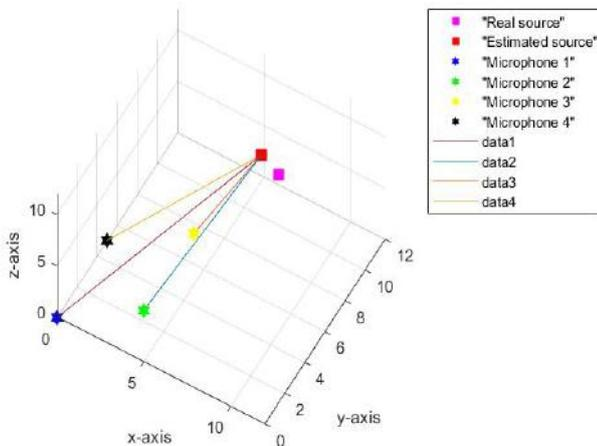
Figure 19. True position – purple color, estimated position-red color, the other colors represents the positions of the microphone
