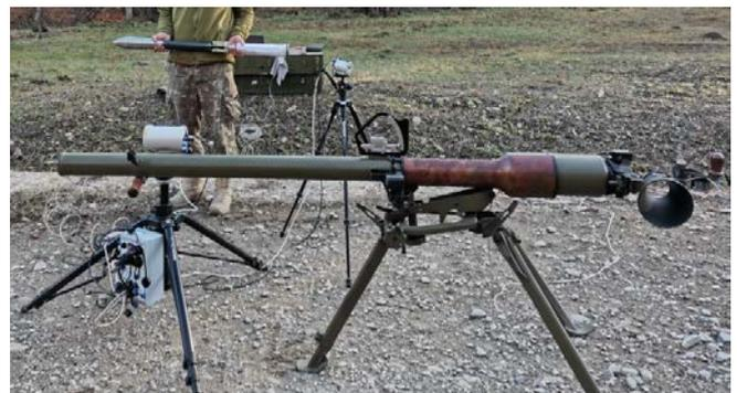
Figure 9. The launcher in firing position with the Doppler radar placed near the barrel and a projectile ready to be loaded
