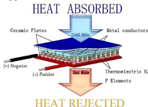
Figure 1. Example of a typical cooler based on TEC technology
