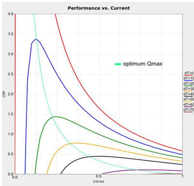
Figure 7. Optimal graph of the correspondence between heat and current supplied for a given temperature difference  $\Delta T$
