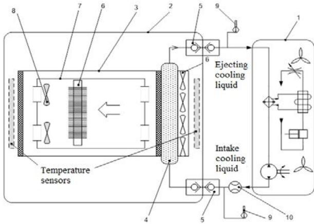
Figure 4. Schematic of the cooling / heating installation in a closed enclosure for a server: 1. Liquid cooling installation; 2. Transport box; 3. RACK TEMPEST; 4. Heat exchanger; 5. Quick couplings connecting liquid cooling system; 6. Heating elements; 7. Model of IT equipment; 8. Mock-up fans of IT equipment; 9. Liquid temperature sensors; 10. Sensor for measuring liquid flow
