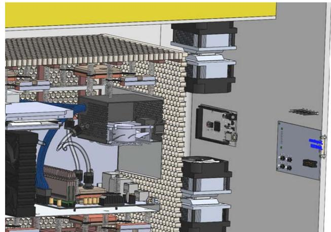
Figure 6. The system as a whole in which the thermal and electromagnetic protection elements for a server can be observed
