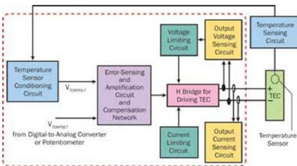
Figure 5. Schematic of the temperature control system based on TEC
