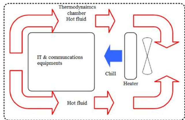
Figure 3. Schematic of the cooling / heating principle in a closed enclosure for a server
