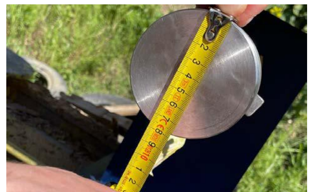
Figure 5. The diameter of the impact surface of the rigid wall
