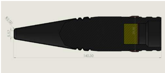
Figure 1. CAD model for projectile equipped with square nose ballistic CAP (section view)
