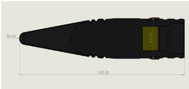
Figure 2. CAD model for projectile equipped with round nose ballistic cap (section view)
