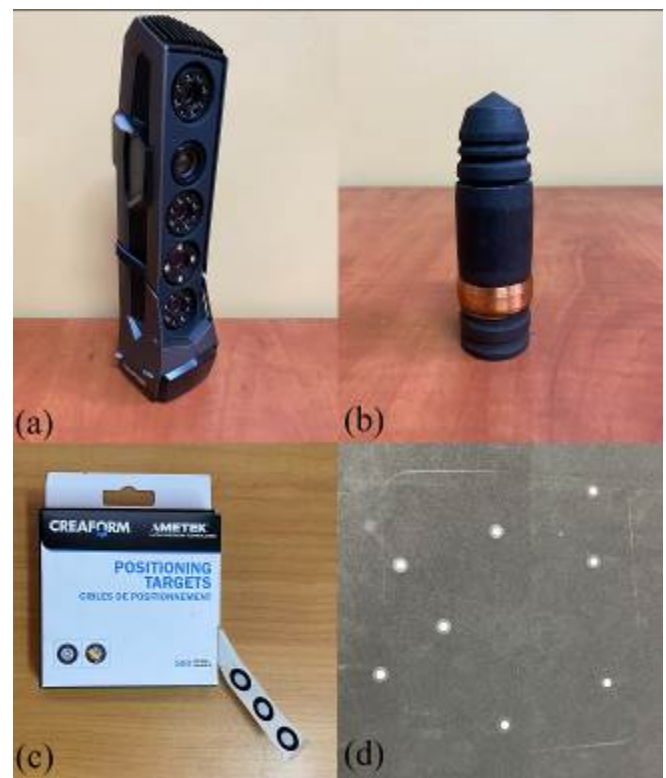
Figure 2. a) Go! Scan Spark 3D Scanner, b) 30×165 mm AP-T projectile, c) Position Targets, d) Surface on which the scan was performed
